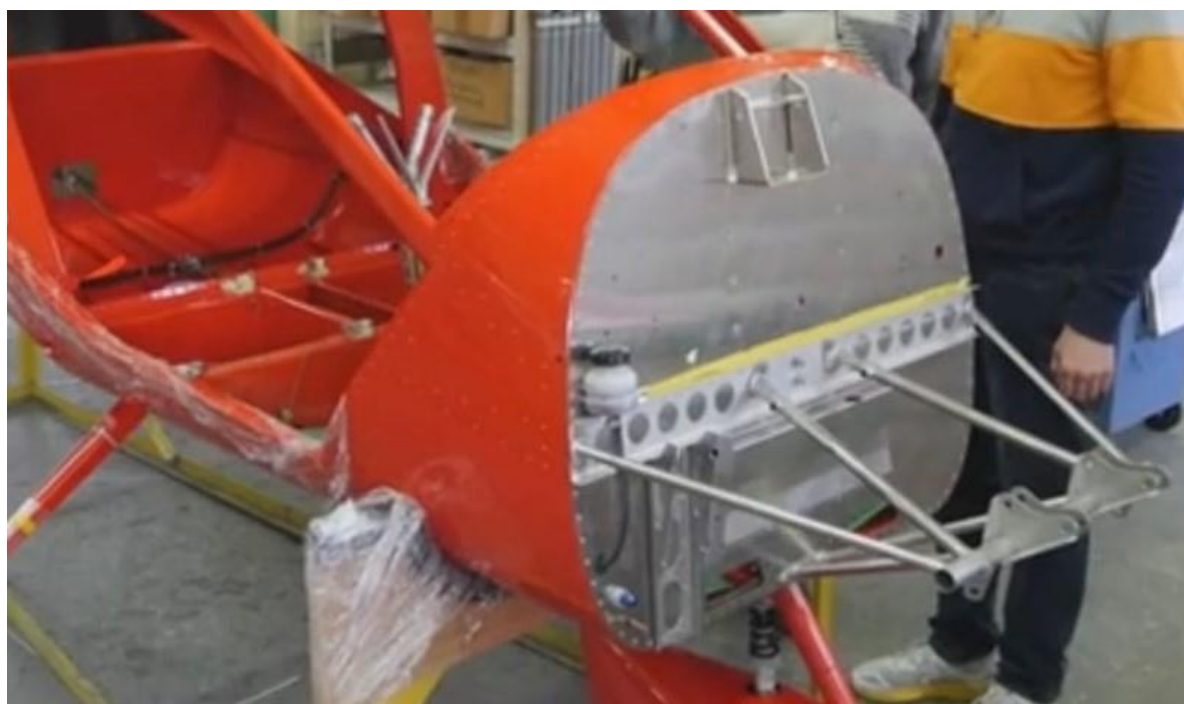
Fig. 2. Attachment points of engine and an example of a mount
